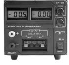
REGULATED POWER SUPPLY WITH VARIABLE OUTPUT a 0-30V, 0 - 3A high quality regulated power supply with variable output voltage and current limiting. The unit has short circuit and "FOLDBACK" overload protection and output is via red (+), and black (-) and green (ground) 4mm terminal sockets. Output voltage and current are indicated by two high precision green LED displays. It is housed in a solid case with power switch.
